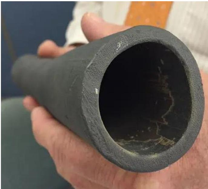
Be sure to scratch-test your pipes in multiple areas. It's not uncommon to have more than one type of piping on your water line.
